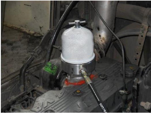
Dieselcraft Oil Centrifuge Model OC-20 on Cummins 24 valve 6 cyl. with universal mounting plate
