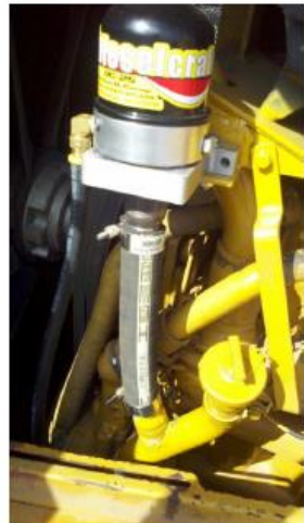
Oil pressure is taken from the "sampling port" on the right side of the engine.
