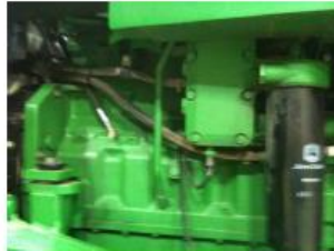
OC 25 Oil Centrifuge on John Deere 9430 Tractor
